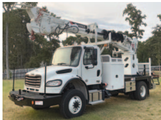
2026 Freightliner M2 Plus 4x4, 360hp Cummins L9, 6-spd Allison Automatic, A/B, A/C, 2012 Terex Commander 5048 Digger Derrick, 25910lbs Max Lift, 48' Sheave Height, Riding Console, Mark IV 2-speed digger head with 18" auger, Pole Claws, 4 Outriggers, Braden PD35A Front Winch, Pole rack, DC to AC inverter ..... $229,350
