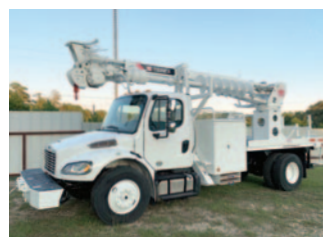
2020 Freightliner M2-106 Utility Truck, 6.7L Cummins, Allison Auto, A/B, A/C, Terex Commander 4047 Digger Derrick, 23660lbs Max Lift, 47' Sheave Height, Riding Console, Turret Winch, Transferable Pole Plummer, 2-speed ESK Digger w/ 18' Auger, 4 Outriggers, Pole Rack, Pintle Hitch..... CALL
