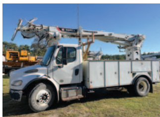
2021 Freightliner M2-106 4x4 Utility Truck, 6.7L Cummins Diesel, Allison Auto, Terex C4047 Digger Derrick, 23660lbs Max Lift, 47' Sheave Height, Riding Console, Pole Guides, 2-spd Digger Head w/ 18' Auger, 4 Outriggers ..... CALL
