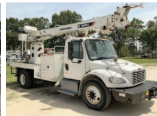
2017 Freightliner M2 Flatbed Utility Truck, 6.7L Cummins, Auto, Terex Commander 4047 Digger Derrick, 23660# Max Lift, 47' Sheave Height, Riding Console, Pole Claws, 2-speed Digger w/ 18' Auger, Pole Rack, 4 Outriggers, Front Winch ..... CALL
