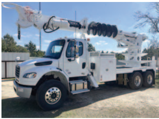
2025 Freightliner M2-106 Plus T/A Flatbed Utility Truck, Cummins 360hp L9 Diesel, Allison Auto, Terex Commander 6060 Digger Derrick, 36000lbs Max Lift, 60' Sheave Height, Riding Console, 3rd FBG/Hyd, 2-speed Digger w/ Auger, 4 Outriggers, Hose Reel, Pintle Hitch ..... $230,500
