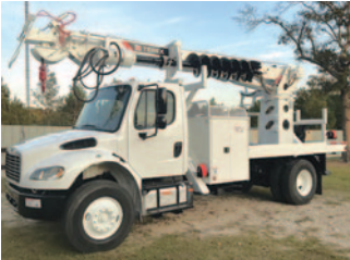
2015 Freightliner M2-106 Flatbed Utility Truck, 6.7L Cummins, Auto, A/C, A/B, Terex Commander 4047 Digger Derrick, 23660lbs Max Lift, 47' Sheave Height, Riding Console, Pole Claws, 2-speed Digger w/ 18" Auger, Pole Rack, 4 Outriggers ..... $87,500
