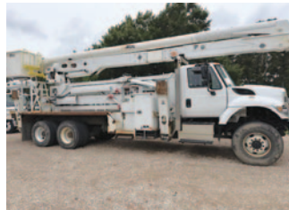
2016 International 7400 6x6 Flatbed Utility Truck, N9 Diesel, Auto, Altec AN67MH-E100, 105' Material Handling Two-Man Bucket, 4 Outriggers. $62,750
