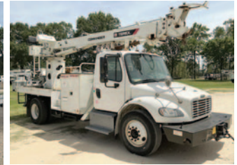
2017 Freightliner M2 Flatbed Utility Truck, 6.7L Cummins, Auto, Terex Commander 4047 Digger Derrick, 23660# Max Lift, 47' Sheave Height, Riding Console, Pole Claws, 2-speed Digger w/ 18" Auger, Pole Rack, 4 Outriggers, Front Winch ..... CALL
