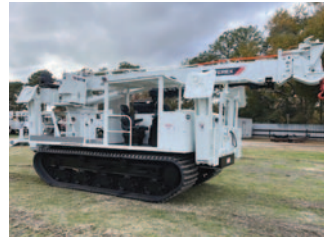
Custom Built LTX180 Rubber Tracked Carrier, 260hp Mechanical 8.3L Cummins, Danfoss Hydrostatics, Terex Commander 5050, 30000lbs Max Lift, Riding Console, 54' Sheave Height, Manual Pull-Out 4th stage, Remote Control, Pedestal Winch, 4 Outriggers, Front and Rear Winch ..... $299,999
