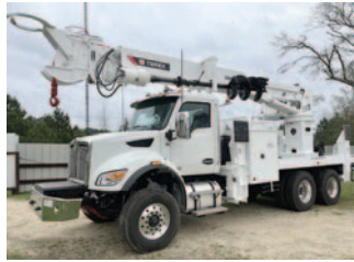
2025 KW T480 T/A Flatbed Utility Truck, Paccar 360hp PX-9 Diesel, Allison Auto, Terex General 65 Digger Derrick, 48000lbs Max Lift, 65' Sheave Height, Riding Console, 3rd FBG/Hyd, 2-speed Digger w/ Auger, 4 Outriggers, Hose Reel, Pintle Hitch ..... $268,500
