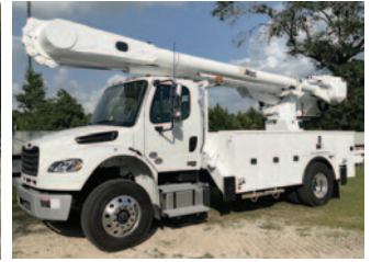
2025 Freightliner M2-106 Plus Utility Truck, 360hp 8.9L Cummins Diesel, 6-speed Allison Automatic, 2015 Altec AM55, 60' Material Handling Two-Man Bucket, 4 Outriggers ..... $190,000
