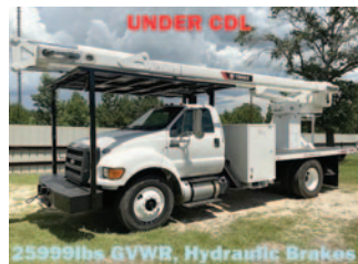
2015 Ford F750 Flatbed Utility Truck, 6.7L Cummins, 6-speed Manual, Hyd Brakes, 25999GVWR, Terex XT60 Rear Mount, 65' Working Height Over-Center Single-Man Bucket, 4 Outriggers, Cab Guard ..... $80,000
